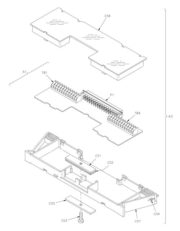
Figure 3-2. Terminal Block Replaceable Parts
