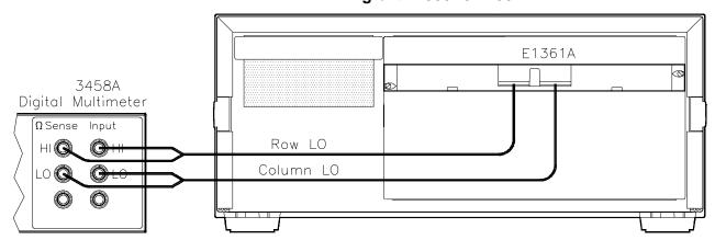
Figure 2-3. LO Resistance Measurement Connections
