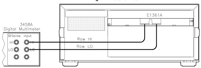
Figure 2-4. HI to LO DC Isolation Connections
