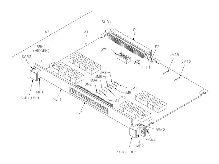
Figure 3-1. Component Assembly Replaceable Parts
