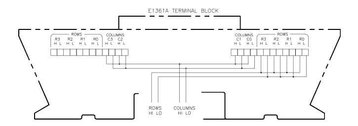
Figure 2-1. Agilent E1361A Test Fixture
