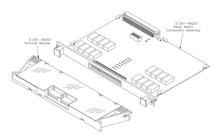
Figure 1-1. Agilent E1361A 4 X 4 Relay Matrix Modules
