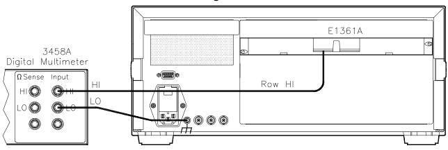
Figure 2-5. HI to Chassis DC Isolation Connections
