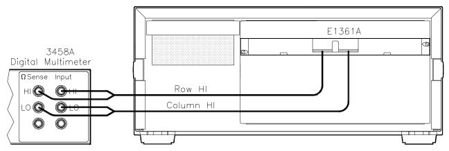
Figure 2-2. HI Resistance Measurement Connections
