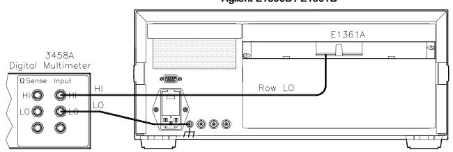
Figure 2-6. LO to Chassis DC Isolation Connections
