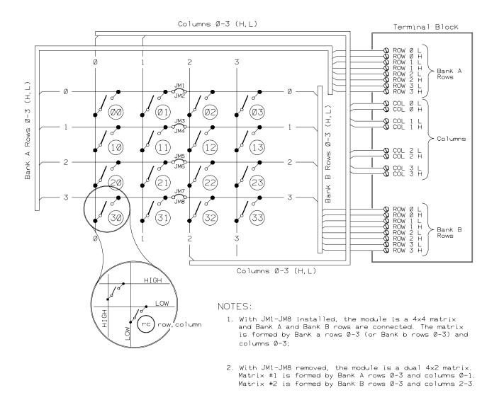
Figure 4-1. E1361A Simplified Switching Diagram
